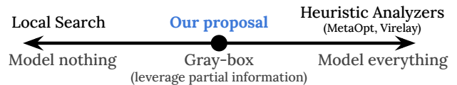
FIGURE 1: We propose a gray-box approach that uses gradient to analyze performance of learning-enabled systems. Existing white-box heuristic analyzers have limited expressiveness and scalability [13, 32, 33] as they require an exact model of the system (including the DNN) in optimization or logic. Local search methods fail to find bad inputs as they ignore all the details about the underlying system.
