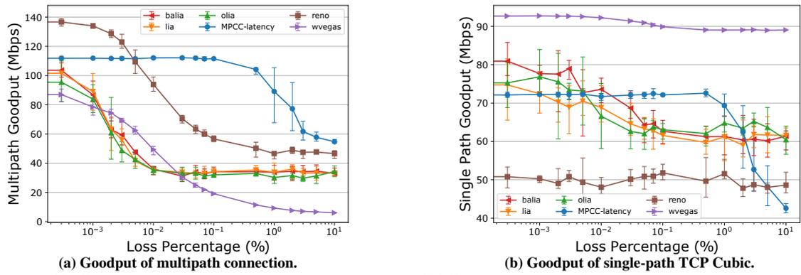
Figure 13: Goodput of multipath sender and single-path TCP Cubic in topology 3c for varying loss rate on link 1
