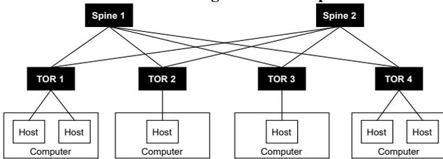
**Figure 18: Our data center testbed topology.**
